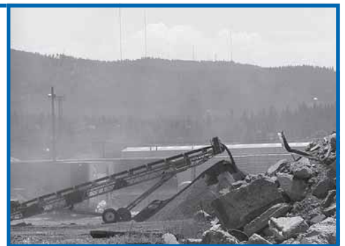
A rock crusher, pictured above, is considered a portable stationary air contaminant source.
